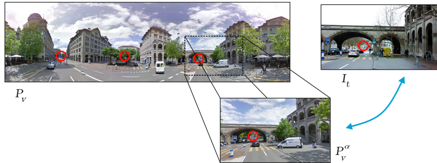
Fig. 3. Street-level vanishing points at an intersection on a panoramic image P_v , and on an image I_t captured by the device. A perspective image P_v^\alpha is extracted for each of the admissible angles, and compared with I_t .
